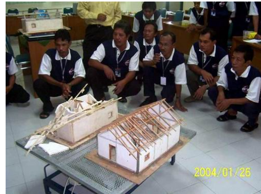
Figure 2: Training mandors (foremen) watch the different behaviour of non earthquake resistant NEHWM and earthquake resistant NEHWM using various simple demonstration tolls, such as small scaled houses on SIMUTAGA SWD-1BM (a simple shaking table) (Sarwidi et. al., 2007)
